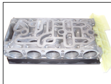
AFTER CLEANING USING NEOKLENE-SONIC 6@ 5% W/W
